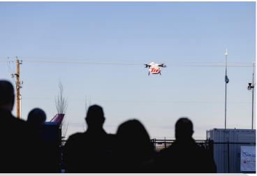
DDC's Sparrow RPA is used for delivering small parcels at a max range of 20km and payload of approximately 4kg.
