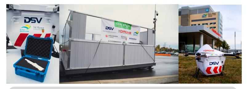
DDC's Sparrow RPA is used for delivering small parcels at a max range of 20km and payload of approximately 4kg.
